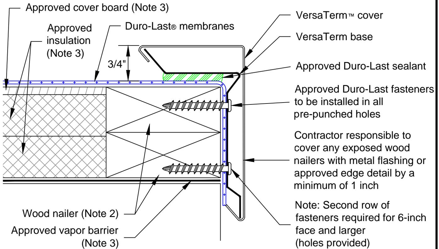
Note 1: Overlap each 10-foot length of base by 1-inch. Overlap the covers by 1-1/2 inches utilizing the pre-notched end on 10-foot lengths.
